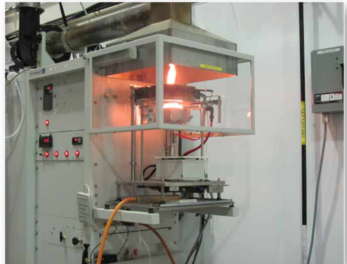
A cone calorimeter is used on site at FPIInnovations. It is a key device used in the field of fire testing to study fire behaviour on sample materials. Photo used by permission of FPIInnovations
